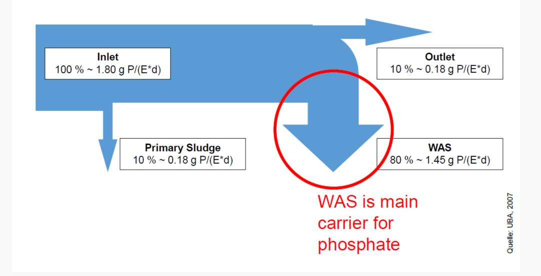
Waste activated sludge from a BNR facility contains approximately:
